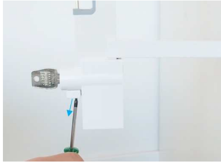
2. Take the screw out from the bottom of the locking slider
