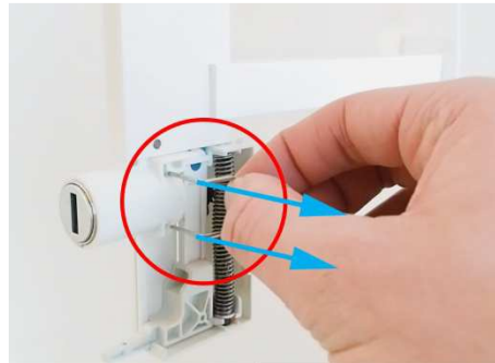
5. Remove the metal circlip
